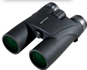
VGV1042 Venture Binoculars DCF. 10x42. Bak4 roof prism. Field of view 98m @ 1000m. Field of view 293ft @ 1000yds. Power: 10. Objective lens diameter: 42mm. Fully multi-coated lens. View angle: 5.6°. Long eye relief: 16.5mm. Near focus: 4m/13.1ft. Diopter adjustment range: ±4D. Waterproof and fogproof. Durable and lightweight body. Emerald
