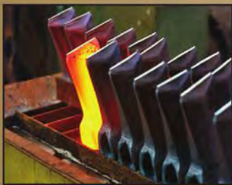
During the process the axe heads are heated repeatedly. This gives the steel superb durability and means a very sharp edge can be achieved.
