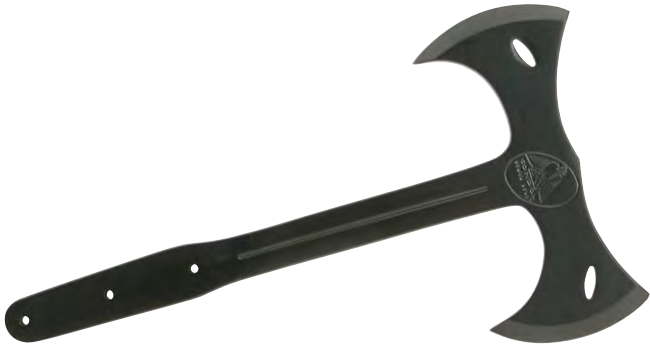
CTK4011BT Double Bit Throwing Axe. 13 5/8" overall. 7" double axe head with 3 1/4" cutting edges. One piece 1075 high carbon steel construction with black epoxy coating. No sheath. .... Retail $49.95
