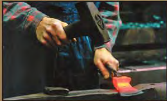
The hammer and anvil are used for the finishing touches. The hands of a blacksmith are still the best tools when producing an axe.
